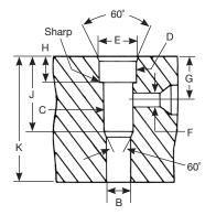
Vacuum Sleeve Chart - 12 sizes available with vacuum passages ("A" diameters) from 3/16" to 2.0".
