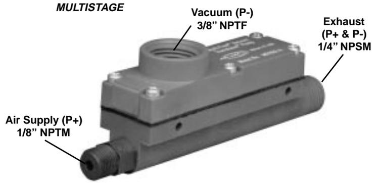
Multistage design with lightweight plastic housing and brass orifice efficiently generates high vacuum flow and high vacuum level. It offers excellent vacuum flow to air consumption ratios.
